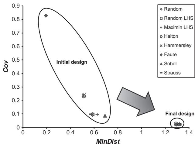
Fig. 3. Comparison of *MinDist* and *Cov* values for eight types of designs. The initial designs ( $N = 3000$  points) present a large variation of the criteria whereas the resulting designs, after WSP selection algorithm ( $N = 400$  points) are equivalent.
