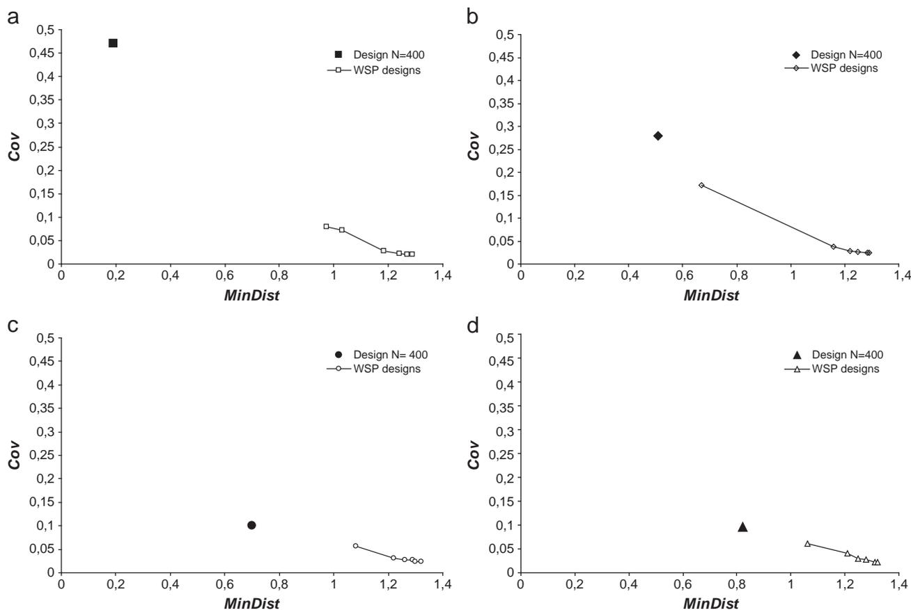
Fig. 4. *MinDist* and *Cov* for designs (*N* = 400 points) after WSP selection algorithm from four initial distributions: random distribution (a), RLHS design (b), Hammersley sequence (c) and Faure sequence (d), with a variation of the number of points in the initial set from 500 to 3000.
