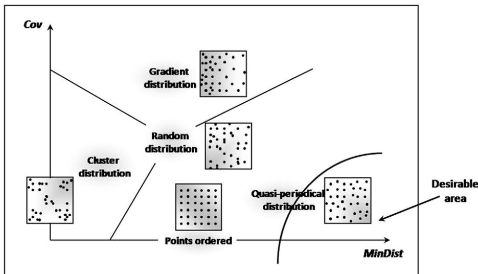
Fig. 1. Empirical repartition of different space-filling designs using  $MinDist$  and  $Cov$  criteria. The desirable designs have a high value of  $MinDist$ , corresponding to sufficiently distant points, and a low value of  $Cov$ , corresponding to a regular distribution.
