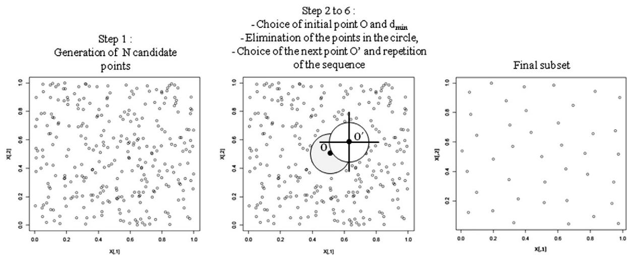
Fig. 2. Illustration of WSP algorithm in 2D space.
